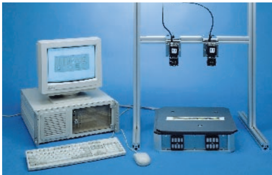
Decal Aligner with Industrial PC and Cameras
