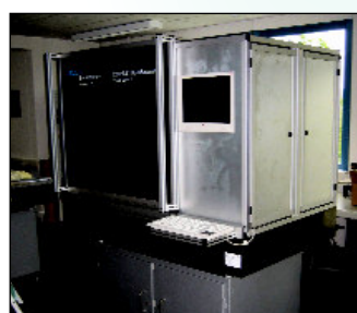
The encapsulated construction enables operation in a shop floor environment
