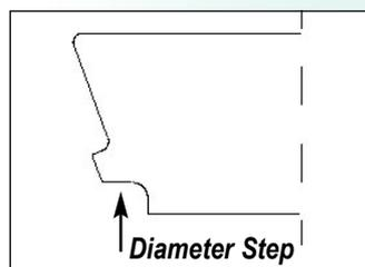
*The roll is in scanning position. At the diameter step the focus can not be in the centre of the roll due to the horizontal plane. Therefore the camera automatically puts the focus on the outside diameter line.*
