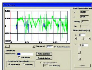
The control of the process reliability postulates the control of the roll forming tools. This can be done fast and easily with the COPRA® RollScanner. If the designed roll is available
