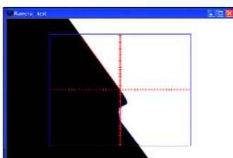
strip guides. Unlike mechanical measuring units that have the limitation of the gauging ball diameter the COPRA® RollScanner is able to measure unlimited small inner radii.
